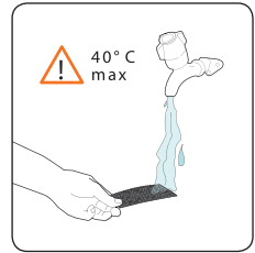
Rinse under water to remove debris (max 40°C).
