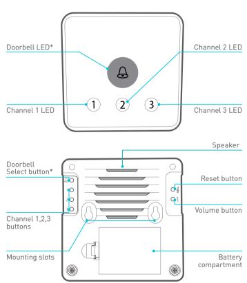
Your Alert Sensor is assigned to channel 1 by default. Each channel is capable of supporting up to 15 sensor devices at a time. Features denoted with \* require separate purchase of an add-on Doorbell.
