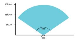
For best coverage and to maximize detection, place the Alert Sensor approximately 2m/6ft off the ground, pointing on a slightly downwards angle.
