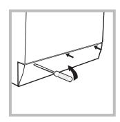
1. using a screwdriver, remove the cover panel on the lower front part of the washerdryer (see figure);
