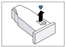
2. Insert the stopper on the underside.
